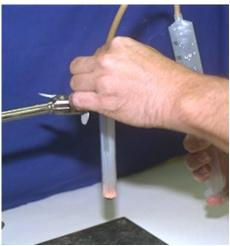
Use the syringe equipped with the tubing/glass pipet attachment to direct the  $Cl_2(g)$  gas in 5 mL increments over the molten sodium from a distance of about 1 cm. A bright, vigorous and short-lived reaction will result. The syringe helps control the direction and delivery of the chlorine gas. The process can be repeated in 5 mL increments of  $Cl_2(g)$  until all of the gas has been used. The reaction is:
