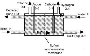
enters the anode chamber where the chloride is oxidized to chlorine:
