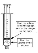
7. Oftentimes during the reaction the plunger does not move as freely as it should and erroneous final volume readings could result. In order to eliminate this problem, draw the plunger outward to create a reduced pressure and then remove the syringe cap under water, using a large container such as an ice cream pail in order to
