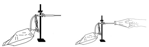
Figure 5. The gas bag being used to discharge a flammable gas at a constant rate.
