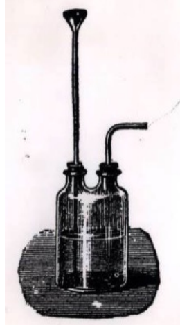
Figure 10. A Wolff's flask. From An Introduction to the Study of Chemistry by Ira Remsen; Henry Holt and Company, New York, 1886.
